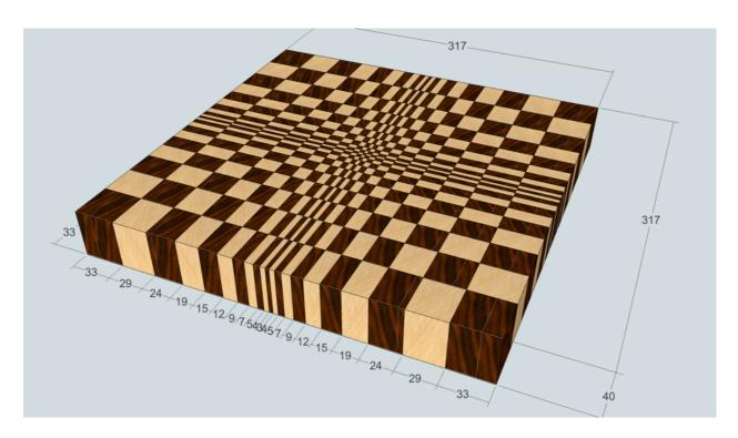
Note that this board is a square. So the dimensions of the appropriate rectangles at all sides of the board are the same.
