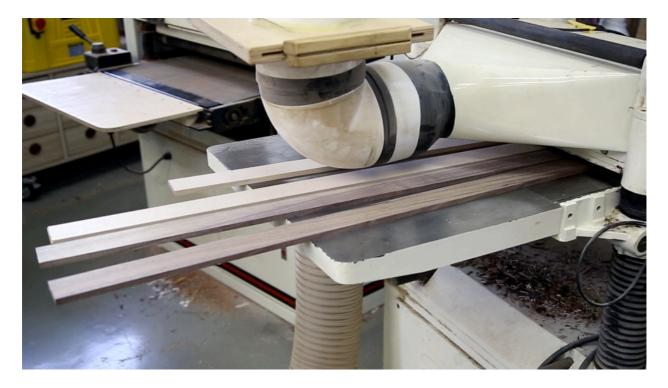
For example, set the level of the planer at 15 mm and plane all four 15 mm strips from two panels at once. The actual thickness may be slightly more or less than 15 mm, but the thickness of all four strips must be the same!
