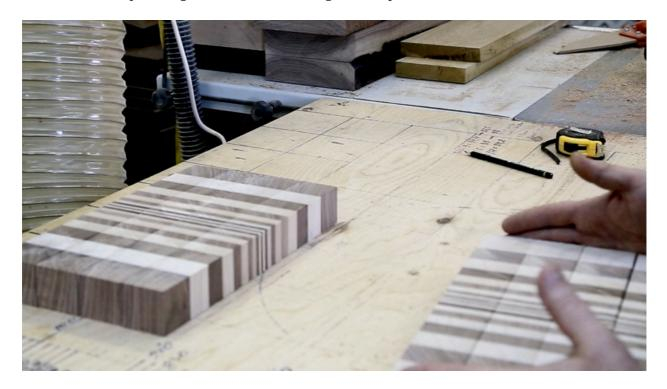
Mark the upper side of the strips and do not rotate them lately. This helps to make a more accurate pattern.
