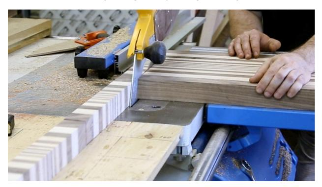
Rotate each strip 90 degrees so that the end grain is up.
