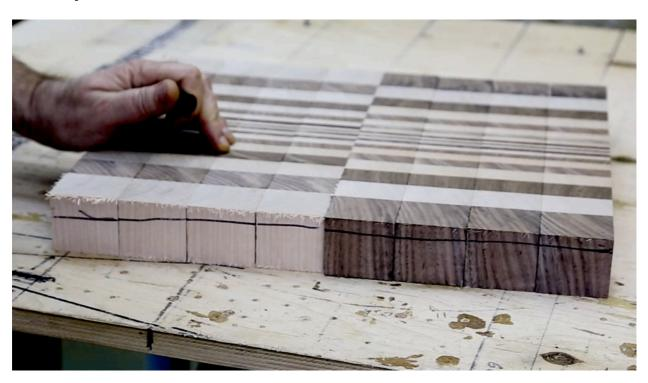
Make the thinner end grain strips at the table saw or band saw according to the drawings.
