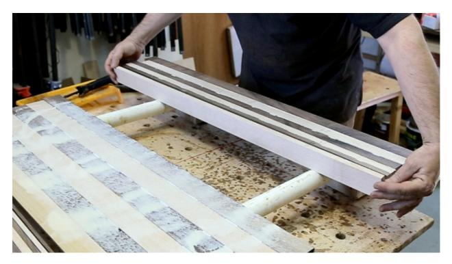
The distance between clamps must be not more than 200 mm.
