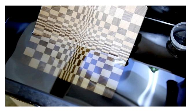
I use a mineral oil bath for 10-15 seconds. Then I dry the board for 6 hours and repeat the oiling.
