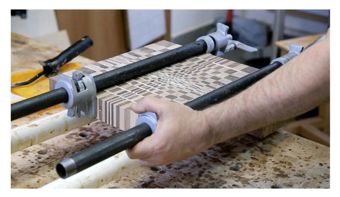
Then turn the board over, place two more clamps and tighten all four clamps with the same force.
