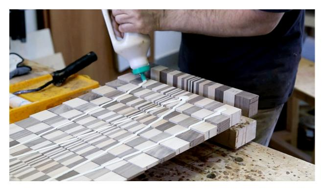
Be accurate assembling the strips. Join the corners of the middle 3 mm maple and walnut rectangles. Control this visually. It is useless to align the strips with the side clamps.
