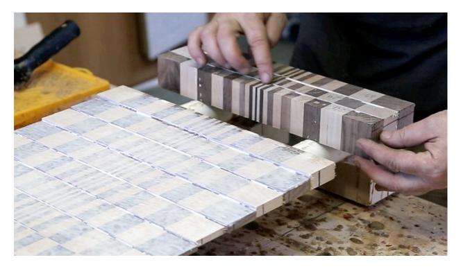
NB! Don't move the strips when clamping! It occurs very often and cannot be corrected. To do this place two clamps exactly perpendicular to the edge of the board and slightly tighten them.
