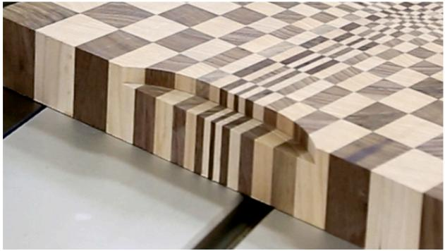
Sand the edges of the board along the grain and slightly round the corners.
