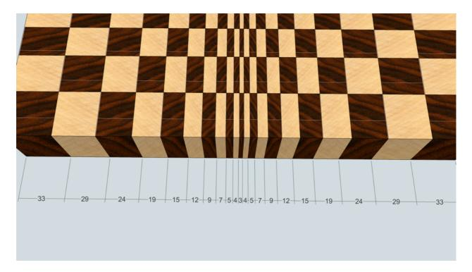
Make the strip thicker 1 mm than in the drawings. You will remove the excess at the drum sander later.
