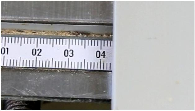
Saw off 42-43 mm wide end grain strips. Usually 4-5 strips are enough to make one board.
